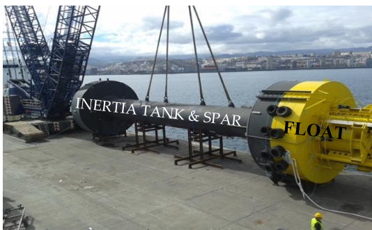
Figure 4. The UNDIGEN Wave Energy Converter proposed by WEDGE GLOBAL a partner of MARES
