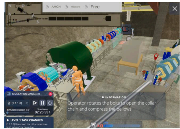
Fig. 4. Screenshot of the HEBT scraper simulation. Manikin simulating worker performing a manual operation.
