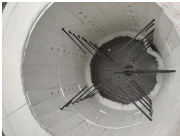
Fig. 3. View and scheme of the interior of the ALTAYR tank with the thermocouples at different locations (no filler in yet).
