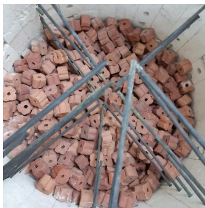
Fig. 4. View of the interior of the ALTAYR tank partially (left) and totally (right) filled with the ceramic pieces used as filler.
