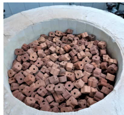
Fig. 4. View of the interior of the ALTAYR tank partially (left) and totally (right) filled with the ceramic pieces used as filler.
