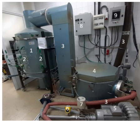
Fig. 2. Picture of ALTAYR packed-bed experimental facility with all its components, adapted from [52].
