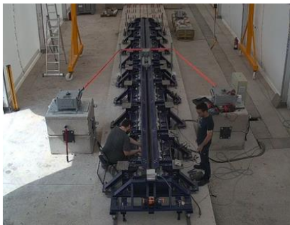
Fig. 20: A real image of the acceleration segment with LSRM that the company Zeleros has at its facilities.
