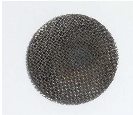
Fig. 5. Gradual porosity 54-38% 310 alloy after test
