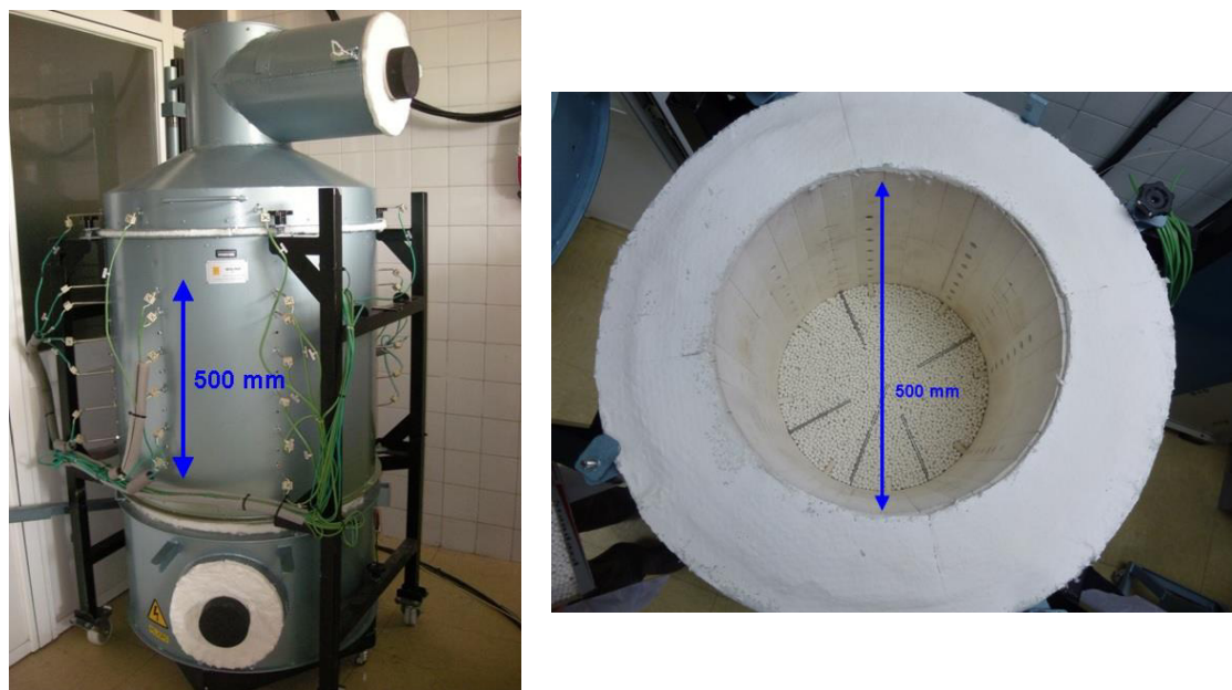
Fig. 1. Packed bed in static arrangement (left), Vessel with thermocouples distribution inside the filler material (right)
