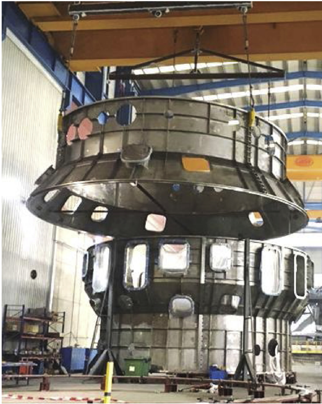
Fig. 5. Assembly of upper sectors on the lower sectors.
