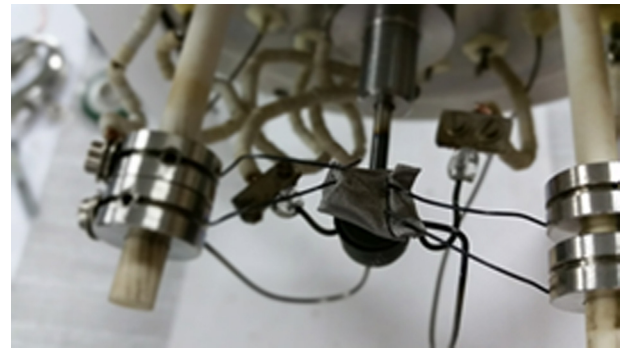
Fig. 2. Set up for the D 2 TID experiments. Pebble samples were contained on the self-made steel bag.
