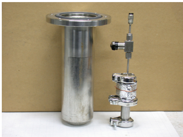
Fig. 1. Pressurized capsule containing the sample load for deuterium sorption experiments under room and gamma-radiation conditions.
