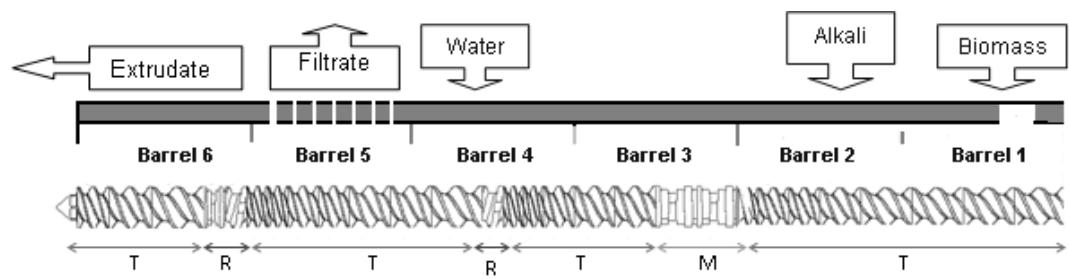
Figure 1. Screw configuration for the extrusion of OTP in the twin-screw extruder. M mixing screw, T: transport screw and R: reverse screw.
