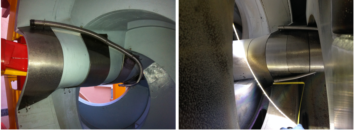
Figure 5. Left: Assembly tests. Piece of supporting corrugated tube positioned inside a 1:1 scale wooden vacuum vessel mockup. Clamps welded to three shaped protecting plates support and guide the tube along the desired path. Right: Final positioning of both helical arrays inside the TJ-II vacuum vessel. Just the initial parts corrugated tubes, starting at \phi = 270^\circ , are seen. The white hanging curved tube is a LED array used for illumination purposes during assembly.
