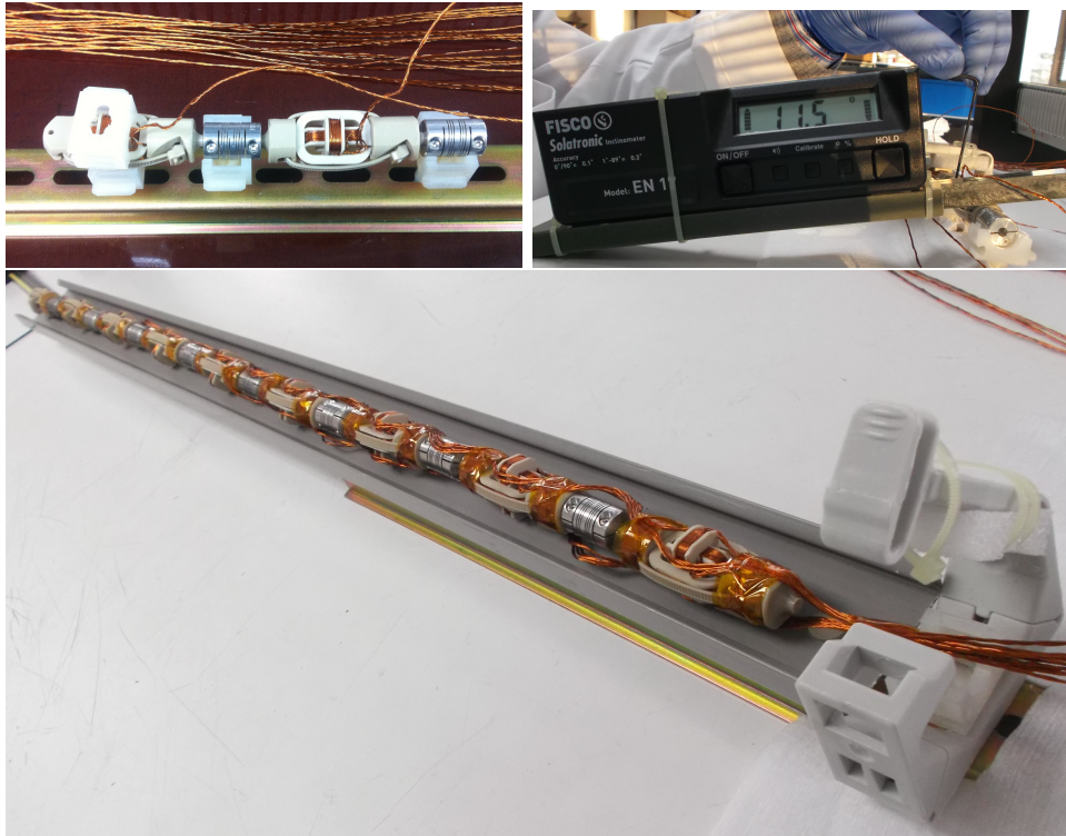
Figure 3. Top left: arrangement of two magnetic sensors and two elastic couplers. Top right: measuring with an inclinometer the required angular twist between adjacent sensors. Bottom: train composed of nine triaxial magnetic sensors with their corresponding couplers in between neighbours. Note the progressively increasing twist imposed to the sensors.
