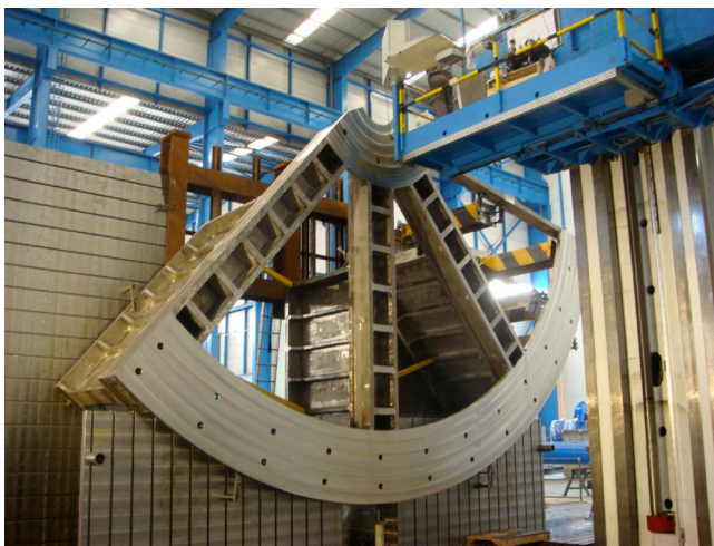
Fig. 5. Lower Structure sector during final machining with the boring machine.
