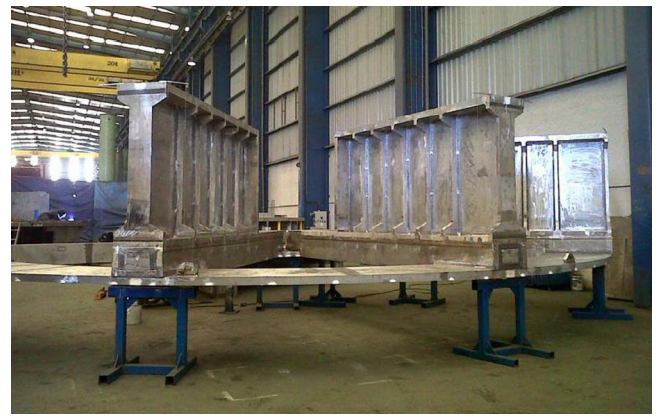
Fig. 3. Lower Structure sector after welding phase.
