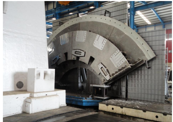
Fig. 6. Double Ring sector during final machining.
