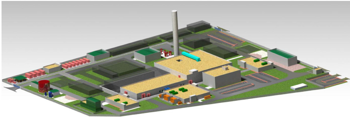
Figure 23. Preliminary layout of DONES in the Granada site (grey buildings are the ones required for a possible future upgrade to IFMIF performance).
