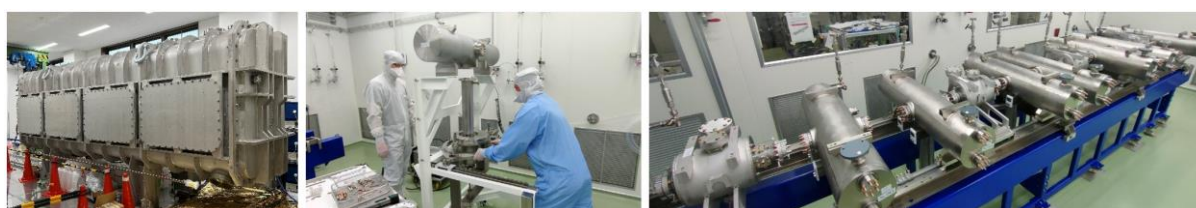
FIG. 9: Vacuum tank of the cryomodule (left), mounting of a cavity in the clean room (middle) and assembly of cavities and solenoids (right).
