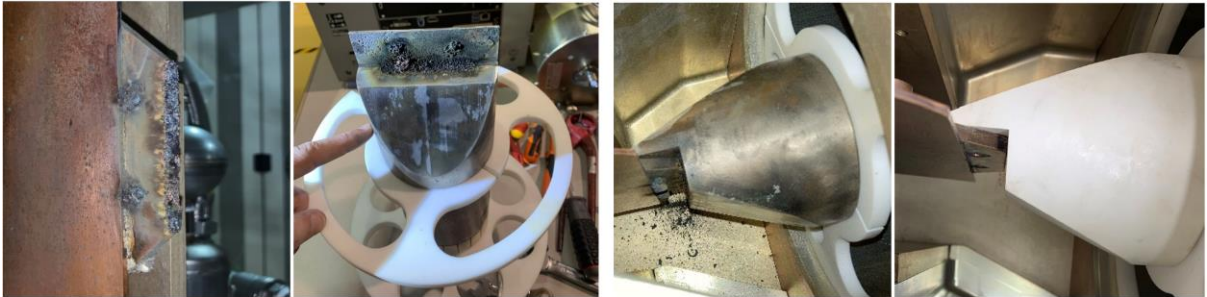
FIG. 4. Circulator 1B inner conductor after onsite inspection and after repair (last right).
