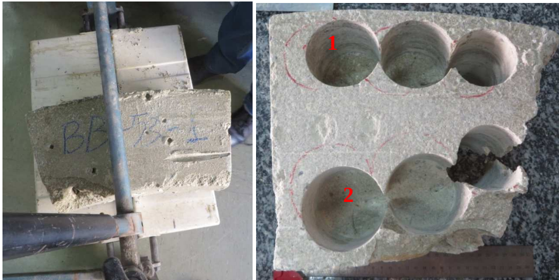
Fig. 14: Sectioning of blocks for THM and THG determinations (left) and drilling of a block to obtain subsamples 1 (closest to the granite) and 2 (closest to the gallery axis) for the HM determinations (right)
