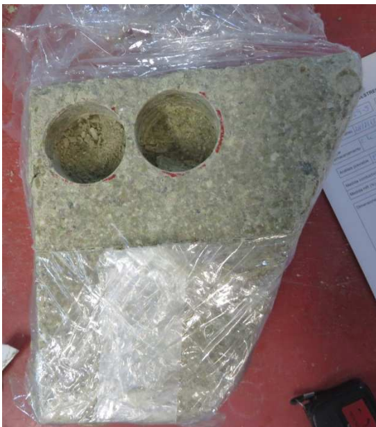
Fig. 22: Appearance of block BB59-5 and location of the two samples trimmed for water retention curves
