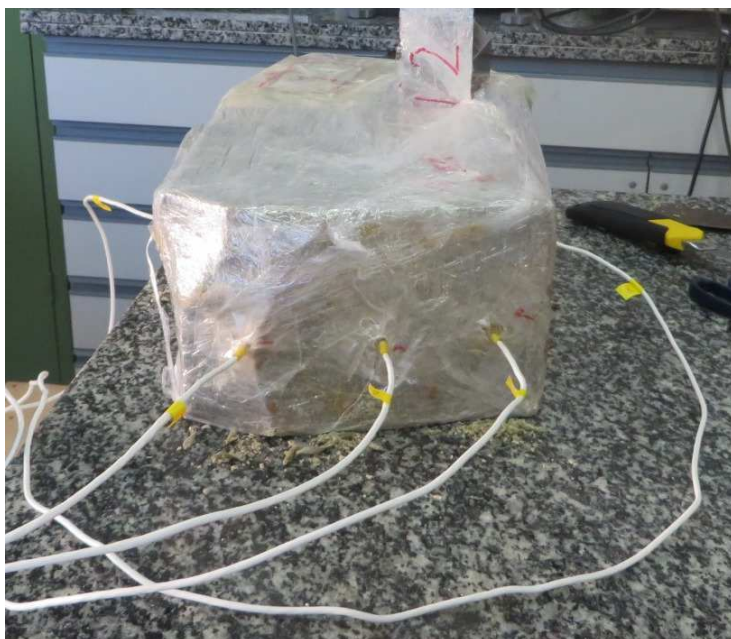
Fig. 15: Psychrometers inserted into a block prior to unpacking
