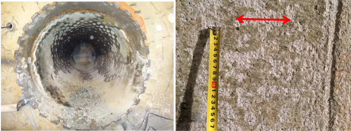
Figure 7: Appearance of the void left after extraction of Heater #2 showing the bentonite intruded through the liner holes (left) and bentonite adhered to granite showing striation parallel to the axis of the gallery (indicated by an arrow, right)
