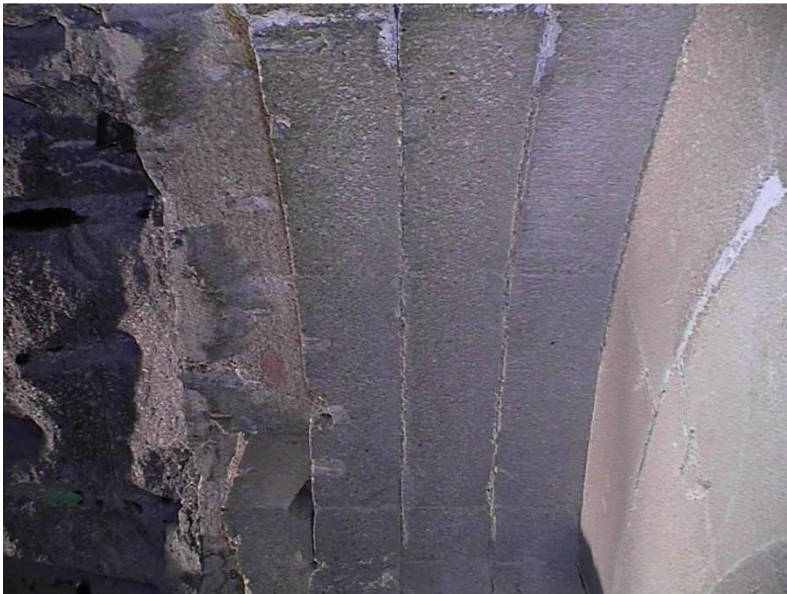
Figure SM-3: View of the external ring of the vertical bentonite slices closest to the gallery entrance during dismantling in 2002. The concrete plug is seen to the left and to the right a non-dismantled bentonite slice
