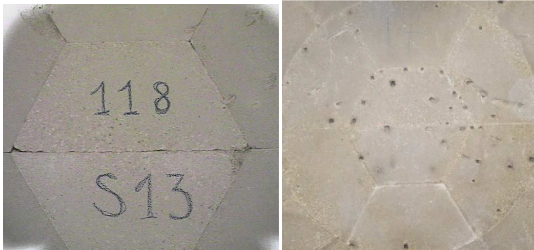
52 Figure 9: Appearance of the core of the barrier in cold zones after 5 years (left, slice 118, section 53 S13) and 18 years (right, slice 17, section S57-S58)
