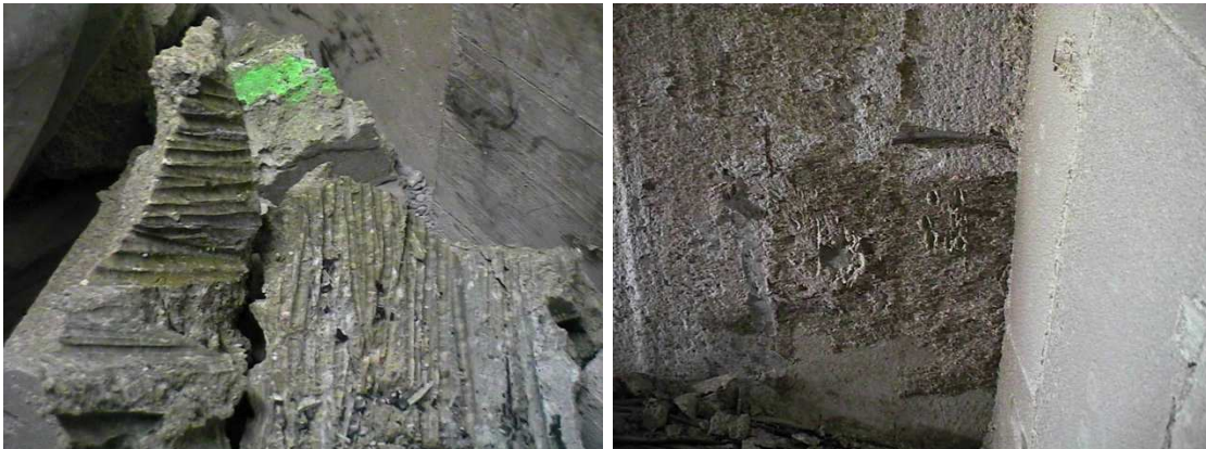
Figure SM-5: Longitudinal grooves on the surface of blocks in contact with granite (left) and bentonite adhered to granite showing striation parallel to the axis of the gallery (right). Photos taken by AITEMIN during dismantling in 2002.
