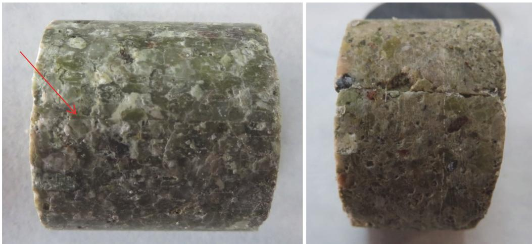
**Fig. 96: Interface in a sample from the external ring (indicated by an arrow, BC-44-6) and from the inner ring (BC-44-2)**
