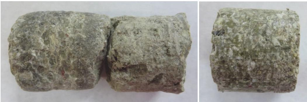
**Fig. 82. Appearance of the core sample BC-53-6 before trimming (left) and after trimming (right)**
