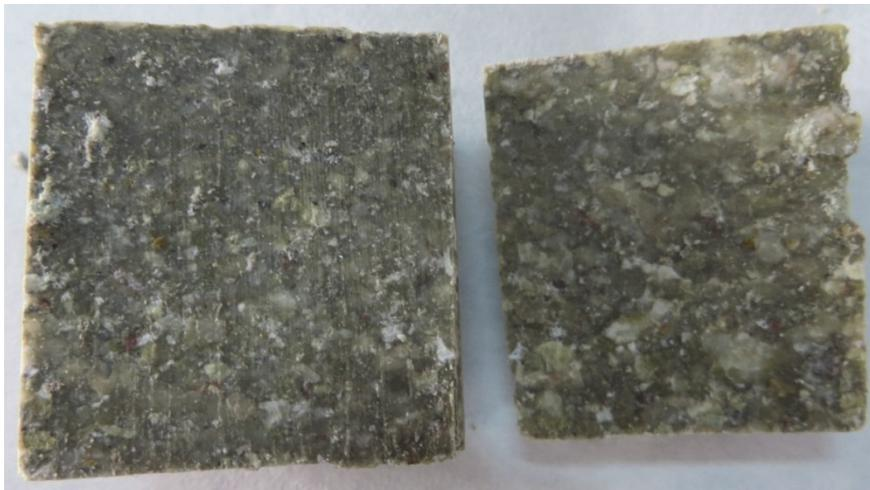
**Fig. 49: Appearance of longitudinal interface of sample BC-47-4**
