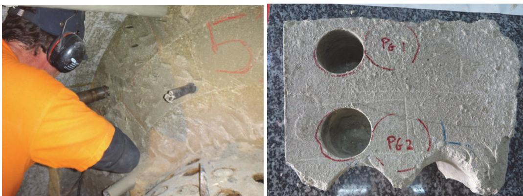
**Fig. 8: Sample drilled on site at the contact between blocks (left) and in the laboratory (right)**
