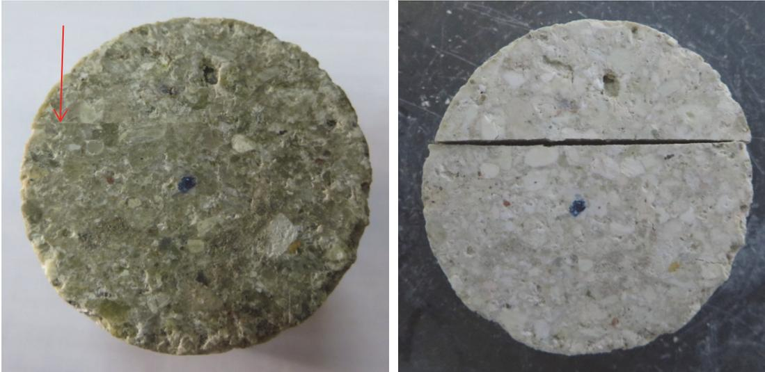
**Fig. 70: Appearance of sample BC-53-2 at the end of gas testing (left, the arrow indicates the interface) and after drying in the oven (right)**
