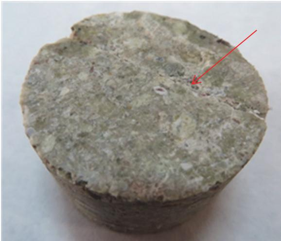
Fig. 27: Final appearance of sample BC-44-2 (the interface can be seen in the upper left)
