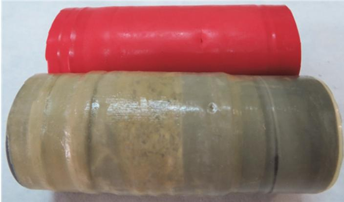
**Fig. 39: Tearing of membrane during testing in the HCP line**
