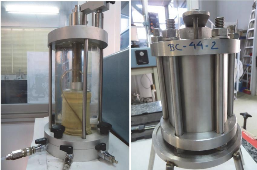
**Fig. 12: Methacrylate triaxial cell (left) and stainless steel high pressure cell (right)**
