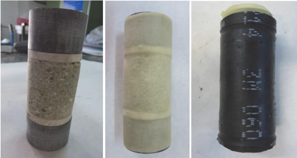
**Fig. 11: Specimen placed between porous stones and perforated PVC discs (left), wrapped in double latex (middle) and latex + EPDM (right)**
