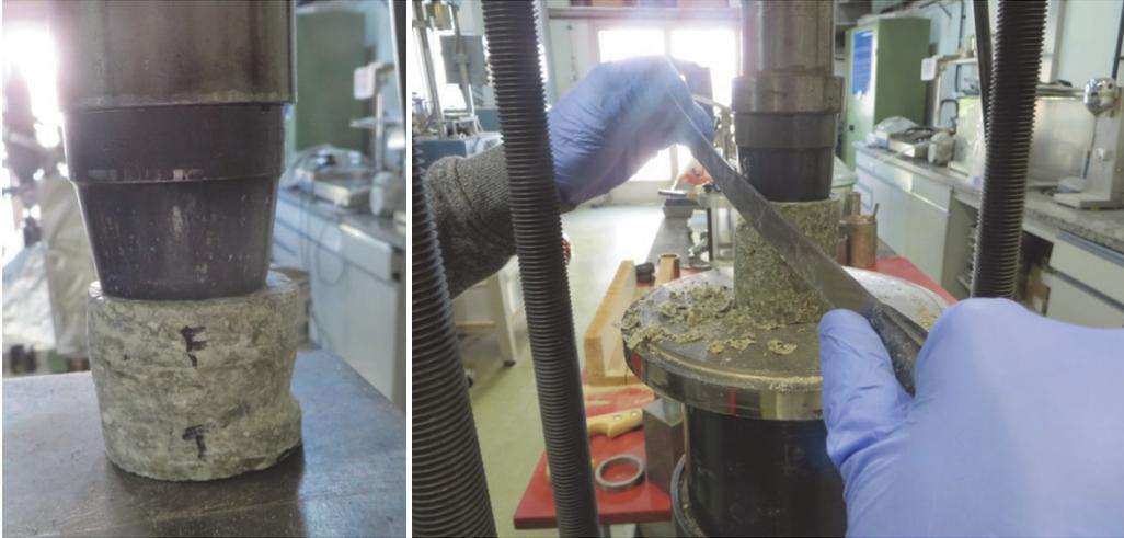
**Fig. 9: Sample preparation: adjusting the diameter**
