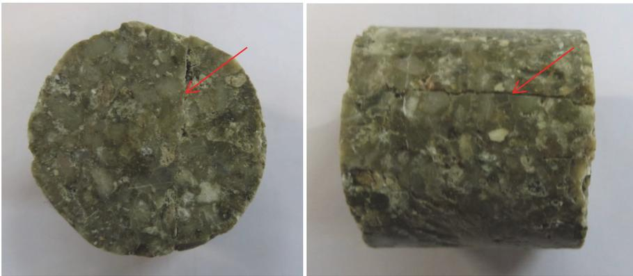
Fig. 77: Final appearance of sample BC-53-4. The arrows indicate the interface after testing
