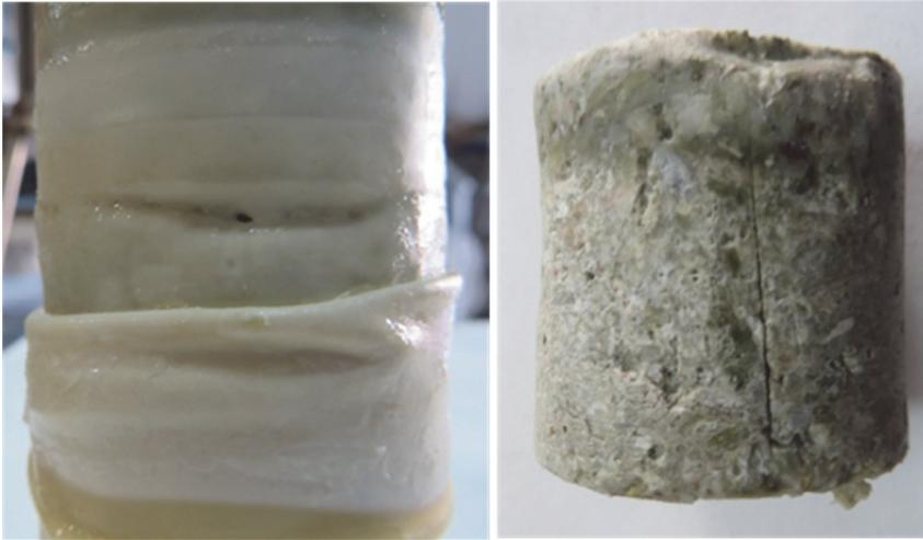
**Fig. 58: Piercing of membranes (left) and appearance of the sample after failure (right)**
