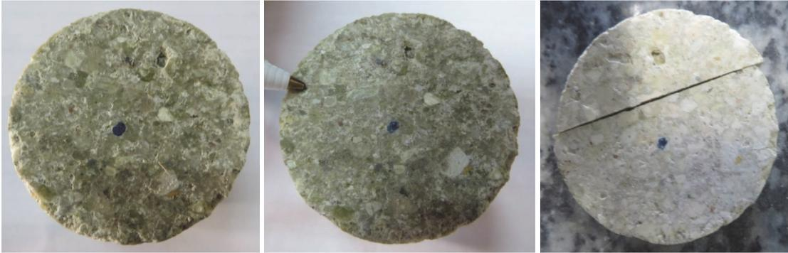
**Fig. 66: Initial (left) and final (middle) appearance of sample BC-53-2. The interface was visible only after drying in the oven (right)**
