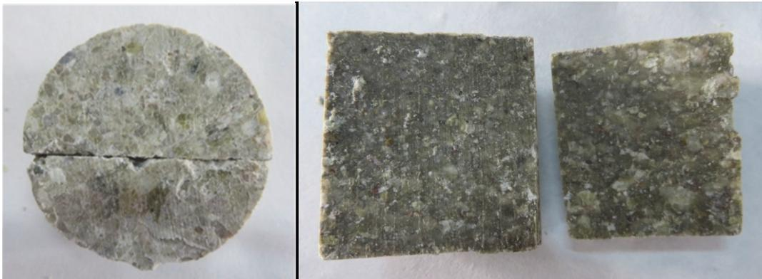
**Fig. 10: Appearance of a specimen prepared for gas test with interface between blocks**
