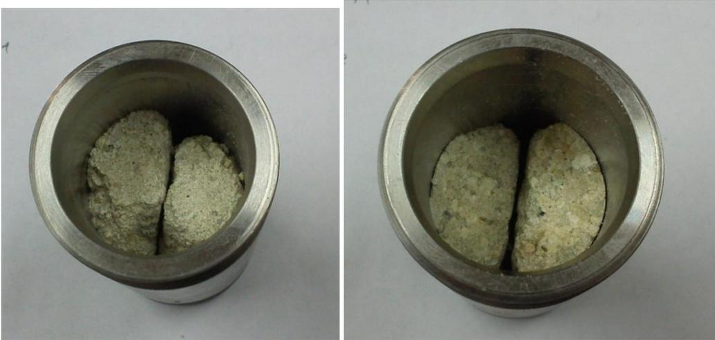
**Figure 9: Appearance of sample BTJ16\_38 prior to saturation inside the cell**
