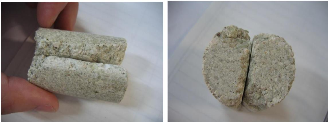
**Figure 8: Appearance of sample BTJ17\_38 prepared for bentonite interfaces testing**
