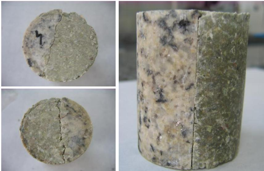
**Figure 66: Appearance of the granite/bentonite interface after the second gas breakthrough in test GB1**
