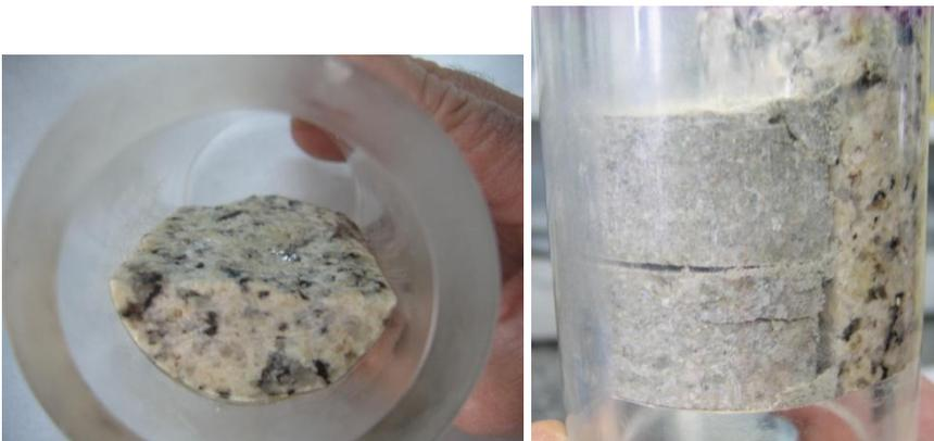
**Figure 10: Preparation of the preliminary test for granite/bentonite interface GB2**
