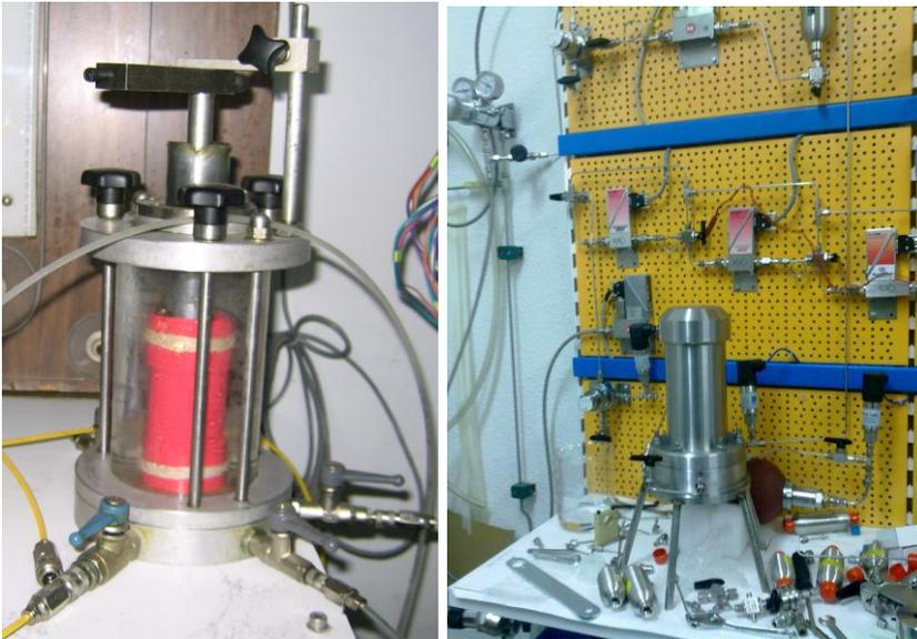
**Figure 1: Bentonite sample inside a methacrylate triaxial cell (left) and high-pressure cell (right)**
