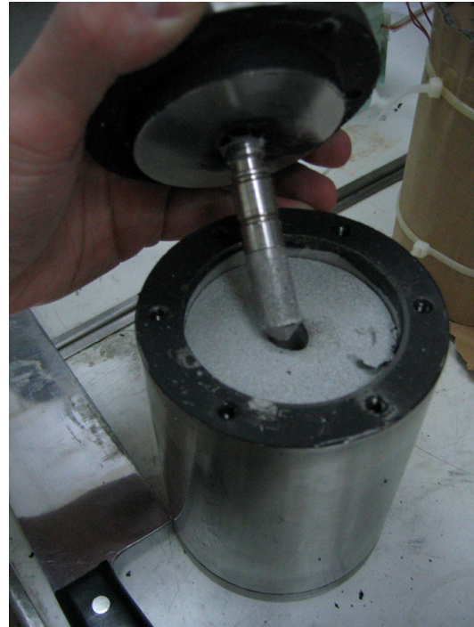
Figure 36: Layout of the cell for the measurement of suction at high temperature with the capacitive sensor inserted in it (dimensions in mm) and appearance of the cell with the compacted bentonite inside, drilled to allow the entrance of the sensor
