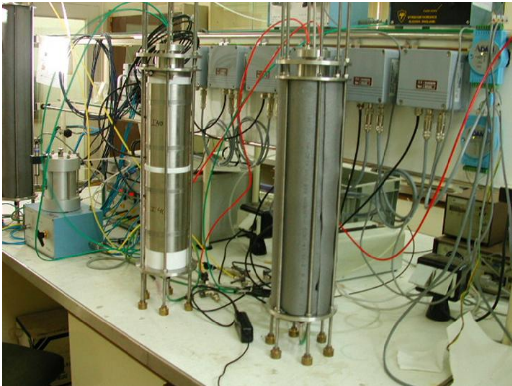
Figure 21: Infiltration cells in operation: isothermal (left) and with thermal gradient (right)
