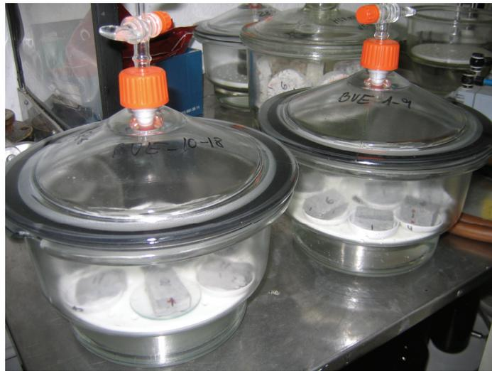
**Figure 9: Samples trimmed from the boreholes, placed in the desiccators**
