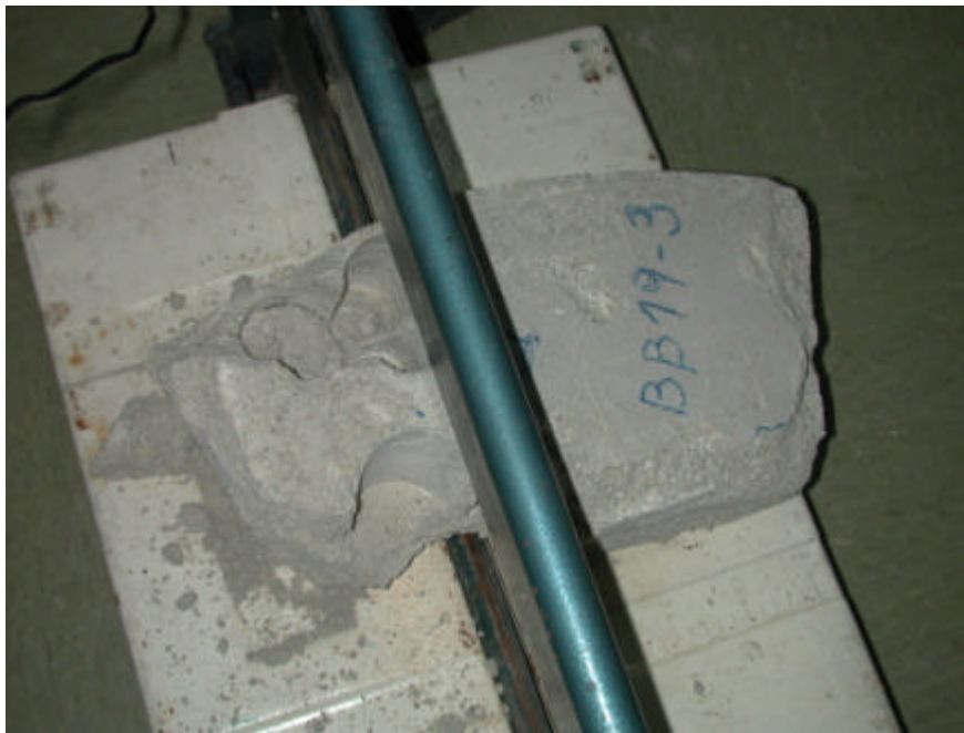
Figure 9: Sectioning of a block for THM (left) and THG determinations (right)
