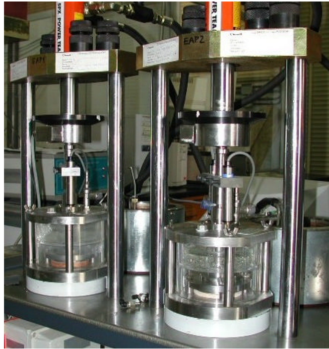
Figure 40: Suction controlled oedometer cells installed in the frames to perform high pressure consolidation tests
