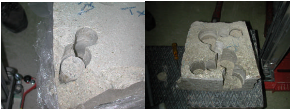
Figure 11: Drilling of blocks to obtain samples for the THM determinations
