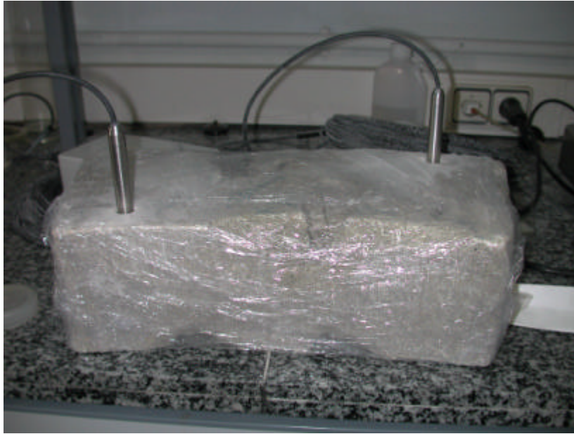
Figure 25: Capacitive sensors installed in two different positions of a block from Grimsel
