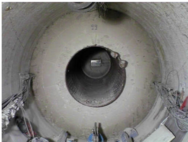
Figure 6: Appearance of the bentonite barrier after extraction of the heater
