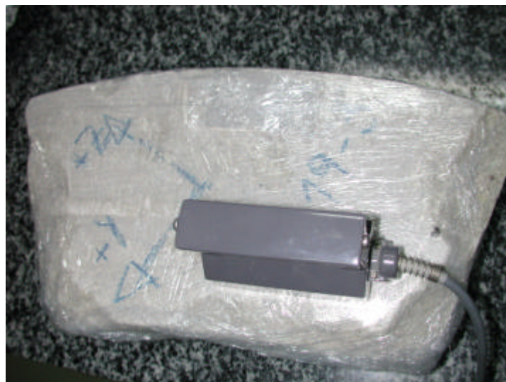
Figure 56: Measurement of superficial thermal conductivity (the plastic foil is removed under the conductivity probe)
