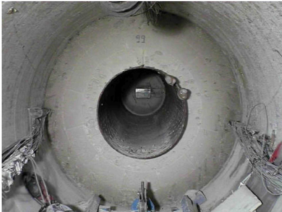
Figure 58: Appearance of the bentonite barrier after dismantling of the first bentonite sections and extraction of the heater in the FEBEX experiment (Bárcena et al. 2003)
