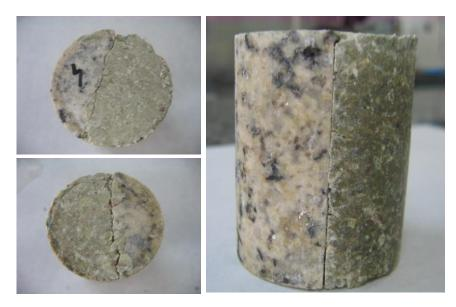
Figure 66: Appearance of the granite/bentonite interface after the second gas breakthrough in test GB1
