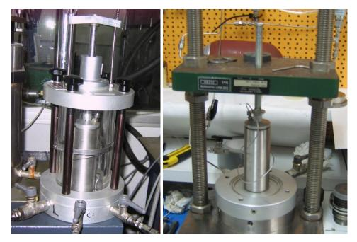
Figure 5: Cell with stainless steel jacket for breakthrough test HP18\_38: during saturation (left) and breakthrough measurement (right)
