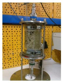
Figure 11: Methacrylate cell during the granite/bentonite interface gas breakthrough test GB1
