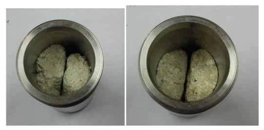
Figure 9: Appearance of sample BTJ16\_38 prior to saturation inside the cell
