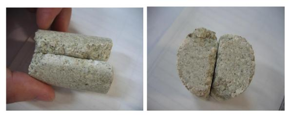
Figure 8: Appearance of sample BTJ17\_38 prepared for bentonite interfaces testing
