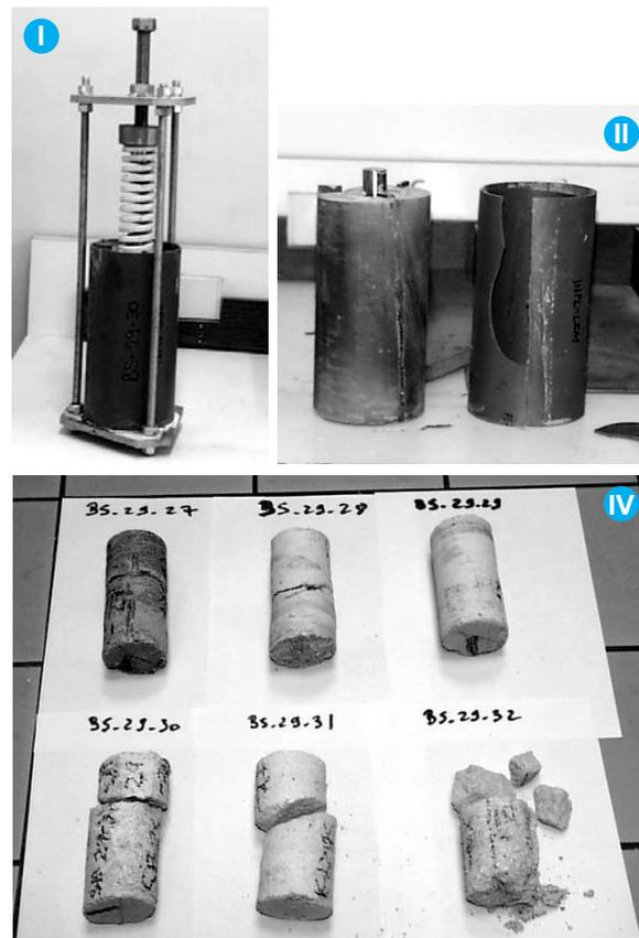
Figure 75: Container (I), opening of the PVC cover (II), appearance of the cores (IV).
