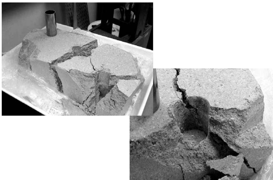
Figure 40: Sampling of a I-doped block by pushing tube.
