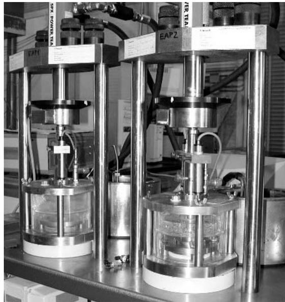
Figure 115: Suction controlled oedometer cells installed in the frames to perform high pressure consolidation tests.
