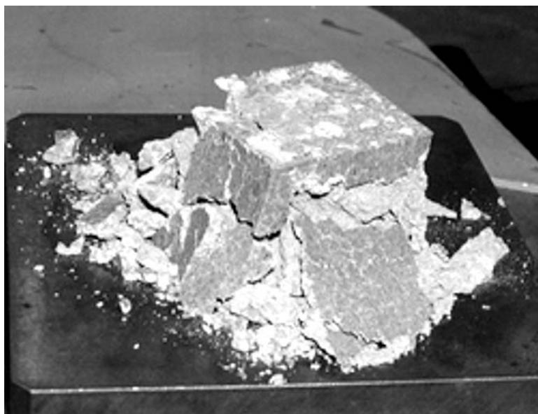
Figure 130: Appearance of a cubic sample after uniaxial strength test.
