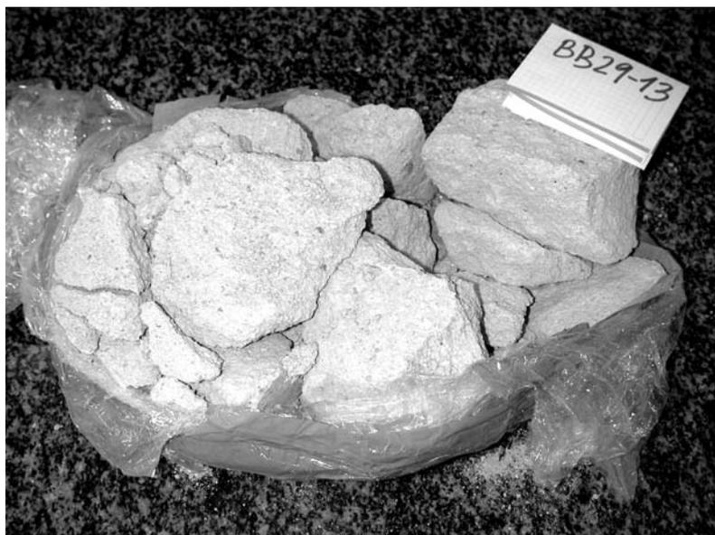
Figure 31: Bentonite block BB29-13.
