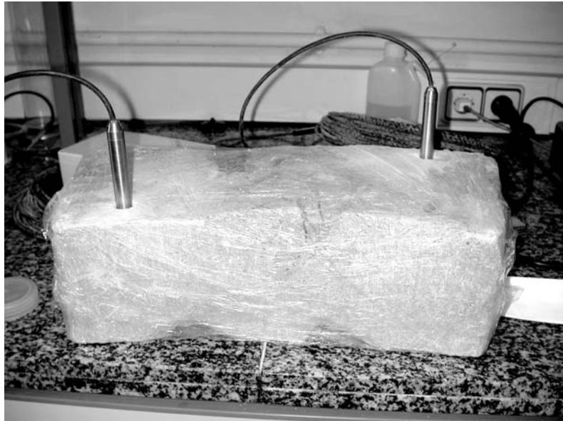
Figure 103: Capacitive sensors installed in two different positions of a block from Grimsel.
