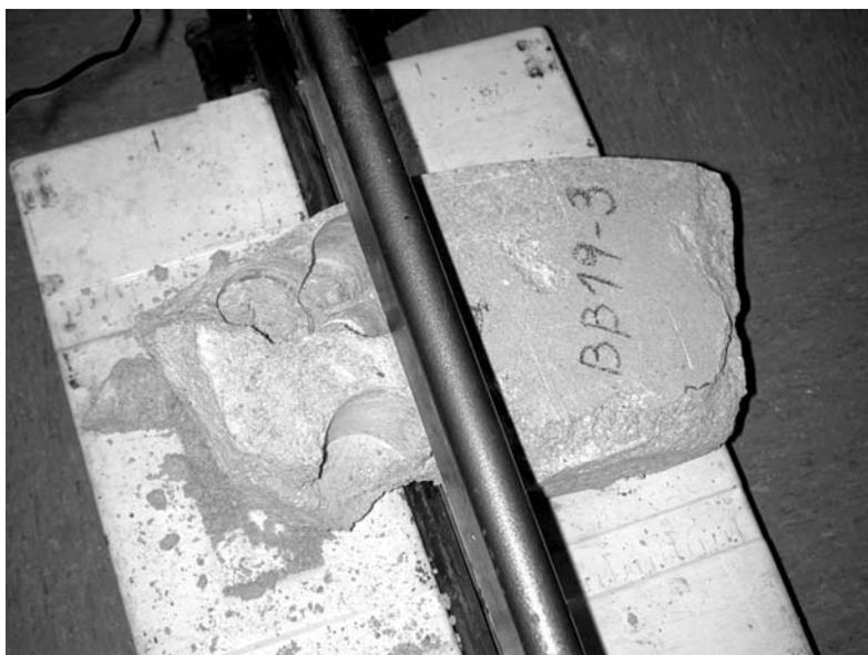
Figure 95: Sectioning of a block for THM (left) and THG determinations (right).
