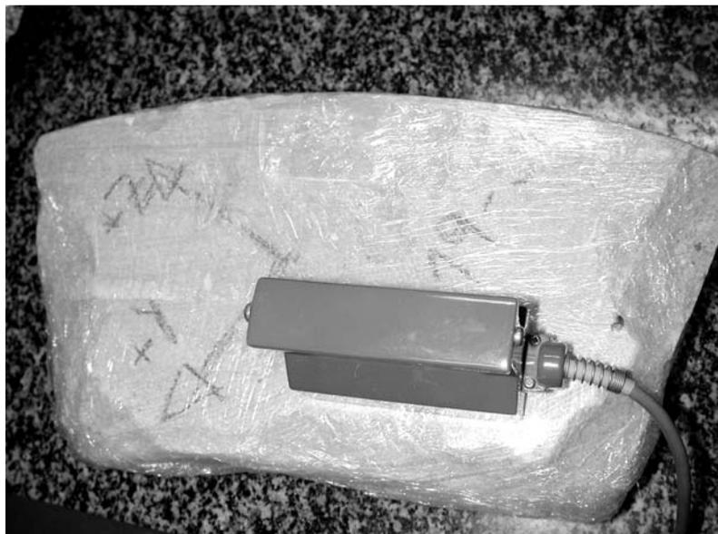
Figure 121: Measurement of superficial thermal conductivity (the plastic foil under the conductivity probe is removed for the determination).
