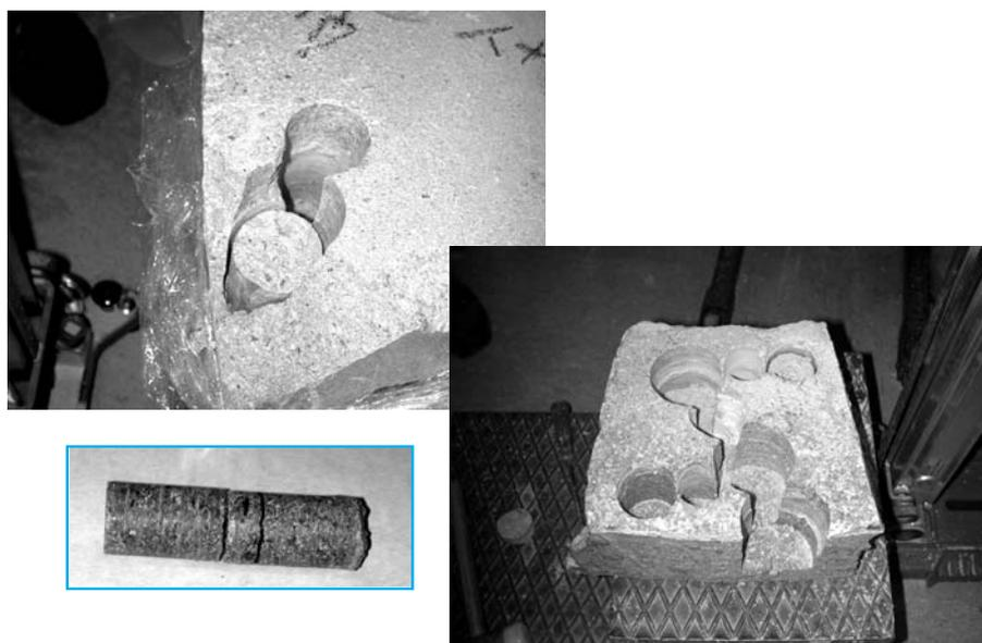
Figure 96: Drilling of blocks to obtain samples for the THM determinations.
