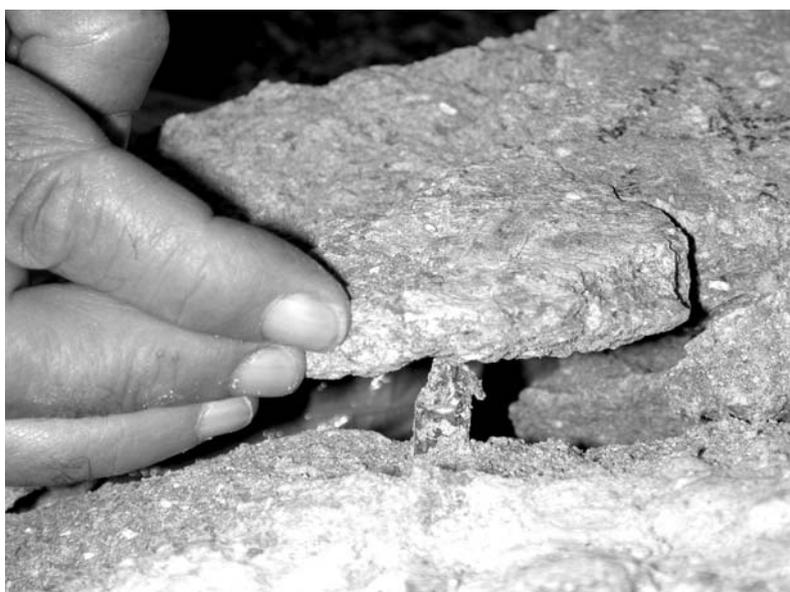
Figure 33: View of the top part of deuterium glass ampoule found in bentonite block BB29-7.
