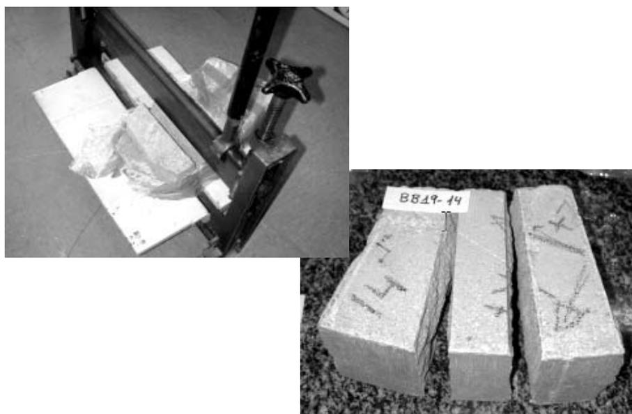
Figure 46. Sampling of blocks for THG analyses at CIEMAT.
