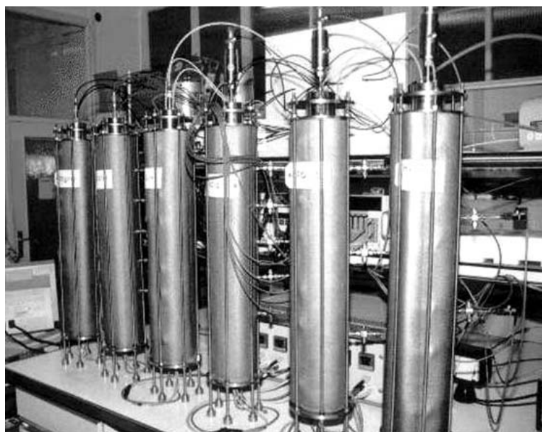
Figure 29: Experimental set-up for the thermo-hydraulic tests (CIEMAT).
