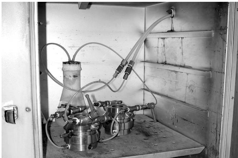
Figure 51: Isochoric cells and salt container to determine the retention curve at constant volume and different temperatures (CIMNE).
