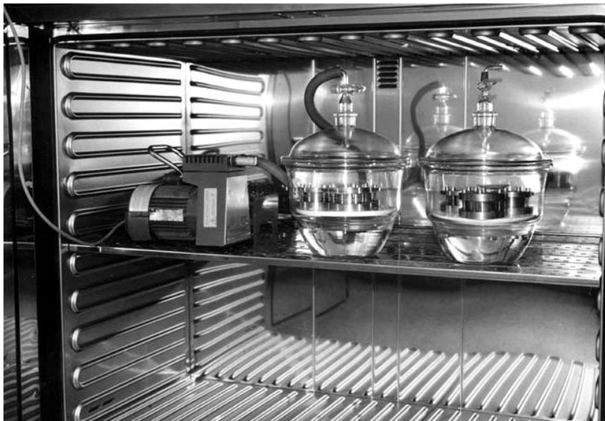
Figure 45: Experimental set-up for the determination of retention curves at constant volume and different temperatures (CIEMAT).
