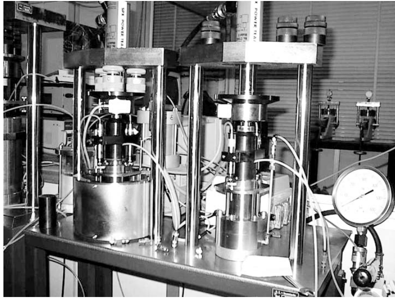
Figure 56: Twin set of high pressure oedometers with one of them placed in the thermostatic bath (left).
