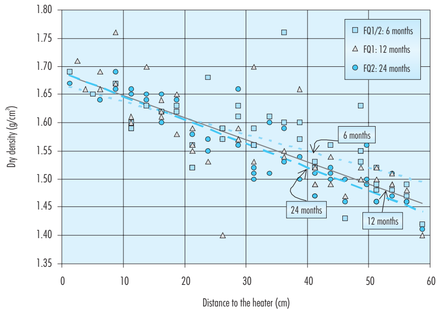
Figure 33: Final distribution of dry density for tests of different duration.
