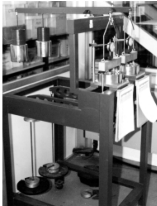
Figure 37. Twin station oedometer frame with cells installed.
