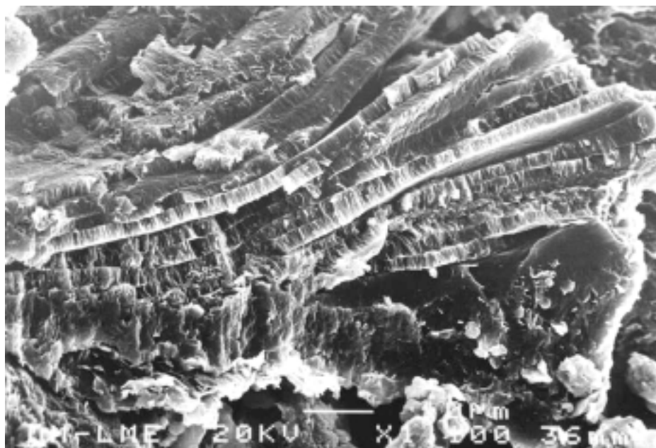
Figure 55. Photograph magnified by 1,100 of the bentonite, taken with the scanning electron microscope.
