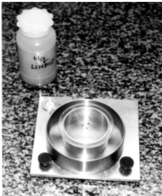
Figure 25. Recipients for the determination of density by immersion in mercury.
