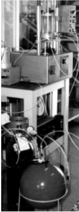
Figure 34. Assembly for measurement of permeability to gas: triaxial cell with specimen, lateral pressure system, gas tank and nitrogen bottle.
