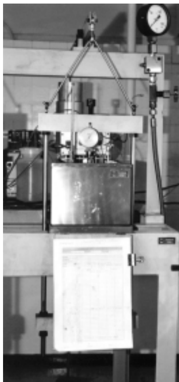
Figure 50. Oedometer with suction controlled by nitrogen pressure installed in a thermostatic bath (manometer to the right, peristaltic pump and water tank to the left).
