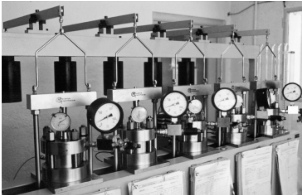
Figure 45. Oedometric frame with five membrane cell stations.
