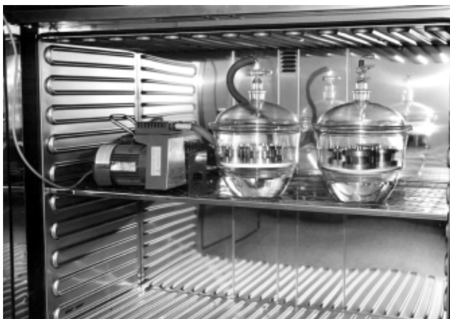
Figure 44. Desiccator with non-deformable cells inside the oven at the moment of vacuum generation.
