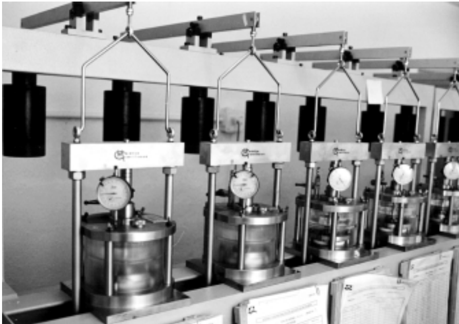
Figure 46. Oedometric frame with five stations for cells with solution deposit.
