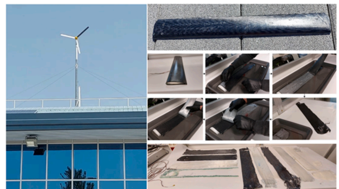
Fig. 4. Process for using glass fibres recovered from recycling to manufacture a second-generation WTB.
