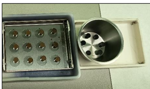
Figure 5. Picture of the \text{UO}_2 pellets sintered with increasing content of \text{U}_3\text{O}_8 .
