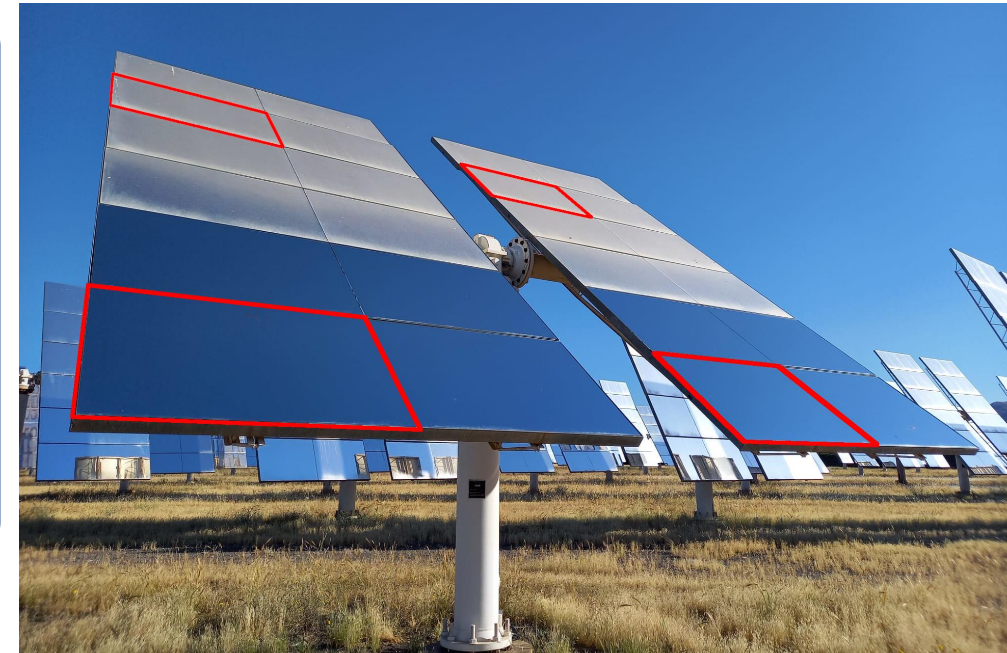
Figure 1: CESA1 heliostat at Ciemat-PSA, Tabernas, Spain, after cleaning lower facets, evaluated facets marked in red
