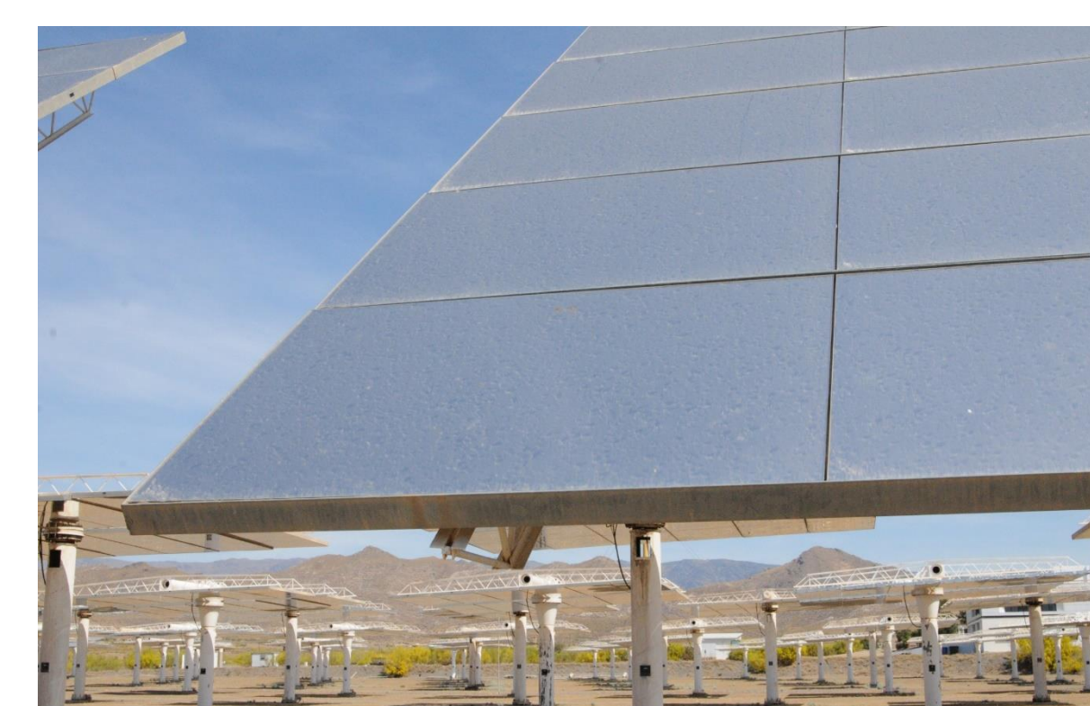
Figure 3: Soiling pattern on one facet after light rain
