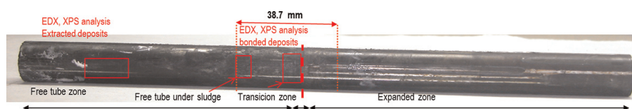
Figure 2. As-reception segment tube. showing deposits analysis areas.
