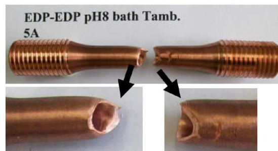
Fig. 8 Typical fracture surface in the joint.
