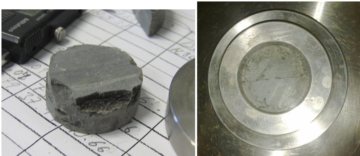
Figure 6: Appearance of samples prepared for the oedometer tests (left: EDS5_F1, right: EDS5_F2)
