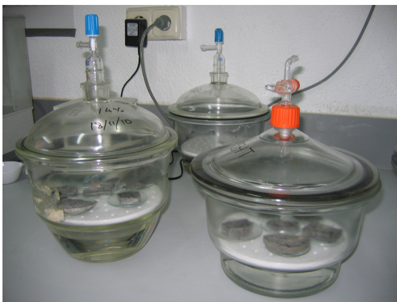
Figure 5: Desiccators for control of the relative humidity
