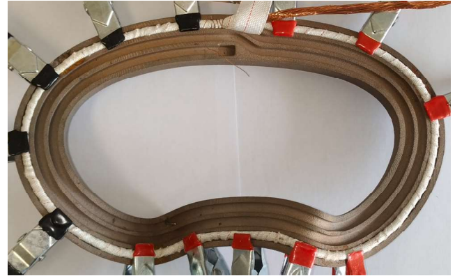
Fig. 9. One turn of variable cross-section flexible copper wire after insulation, inside the groove of the radial plate.
