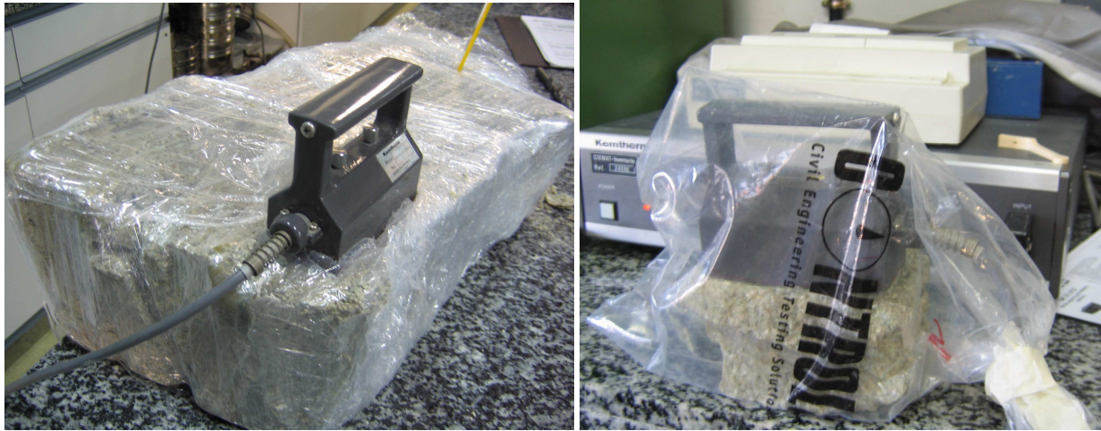
Figure 10: Measurement of thermal conductivity on a bentonite block surface and on a GBM sample
