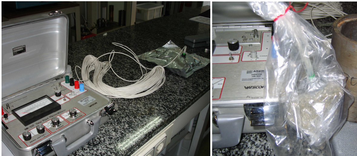
Figure 9: Measurement of relative humidity and temperature with psychrometers
