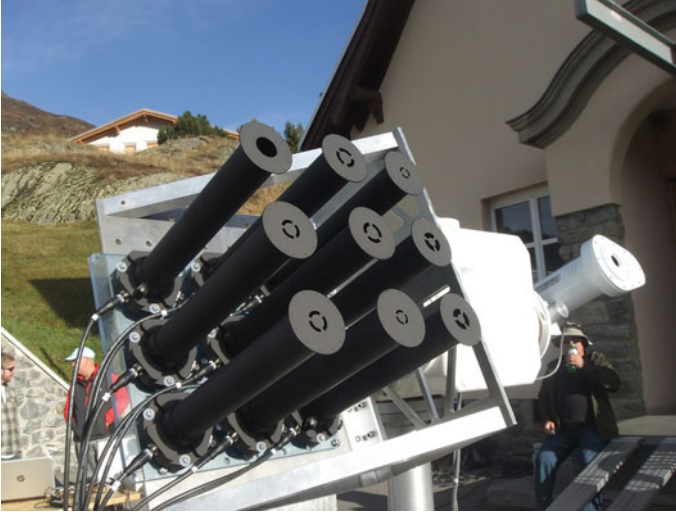
Fig. 16 Measurement of circumsolar radiation from the difference between DNI signal of partially shaded and unshaded sensors during IPC-XII in Davos, performed by Black Photon Instruments
