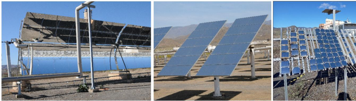
Figure 4. Reflectors used for the measurement campaign: left) PTC, middle) heliostat, right) sample exposure rack.
