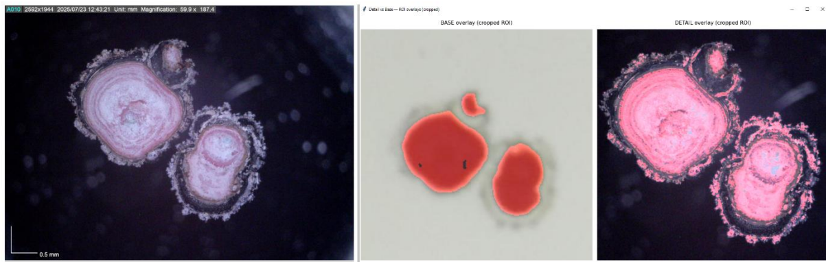
Figure 10. Left) microscopic image of selected corrosion spots of 10x10 cm 2 sample. Middle) zoom of analyzed degraded area on sample image. Right) analyzed area on microscopic image, corrosion marked in red.
