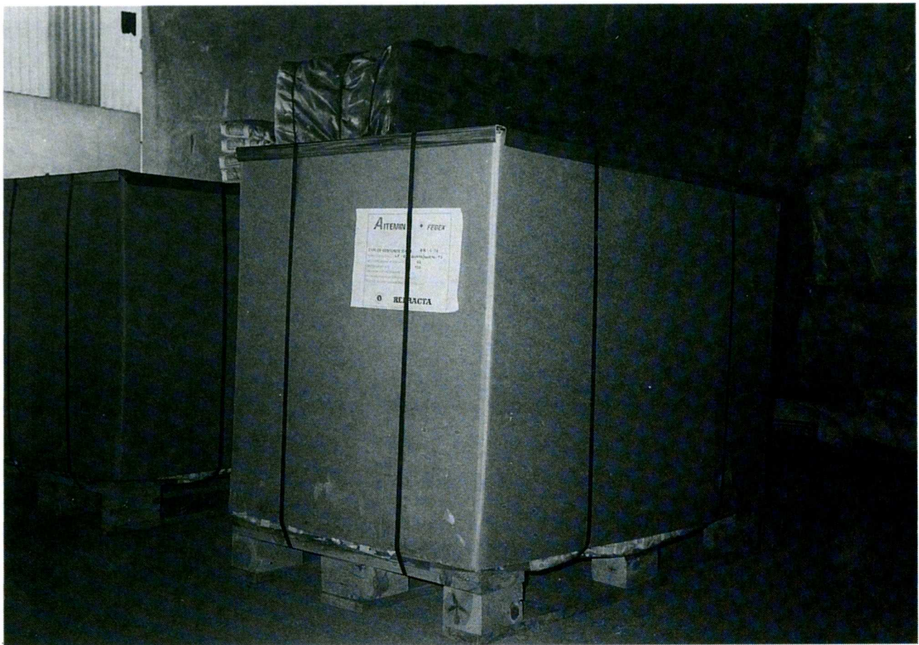
Figure 5.17: Finished package of blocks. Shown are the base of package (pallet), the reinforced corners, the labeling, and the shrink wrap.
