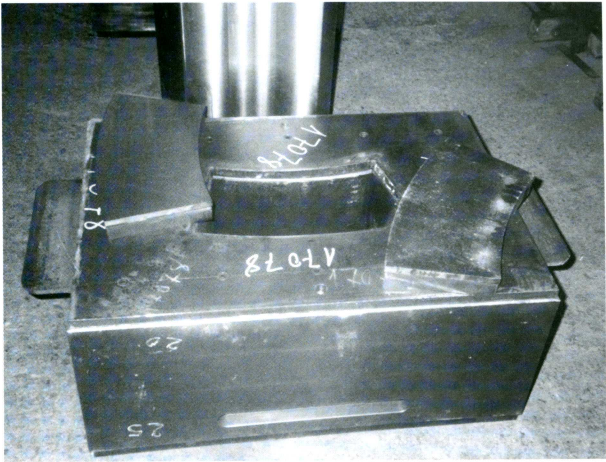
Figure 5.10: View of die of the mold. Over the die are situated two punches of the mold.
