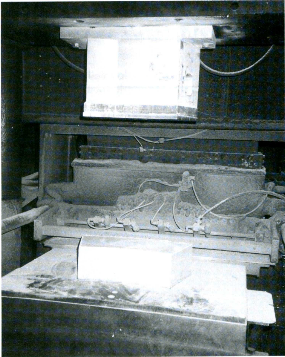
Figure 5.12: Frontal view of the mold installed in the press. In this photo the upper punch is in stand position and the lower punch (not shown) is at the high of the upper face of the die (press table), supporting the bentonite block which has just been compacted.
