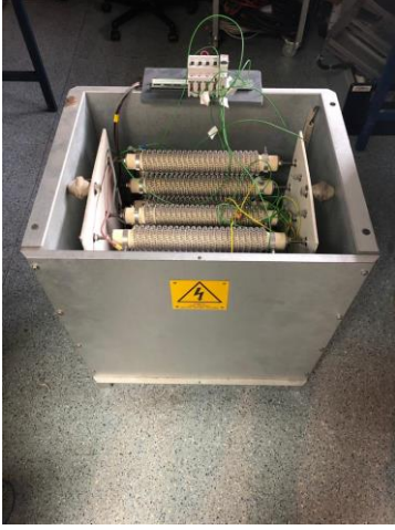
Fig. 12. Resistive load [ R_{phase} = 50 \Omega ].
