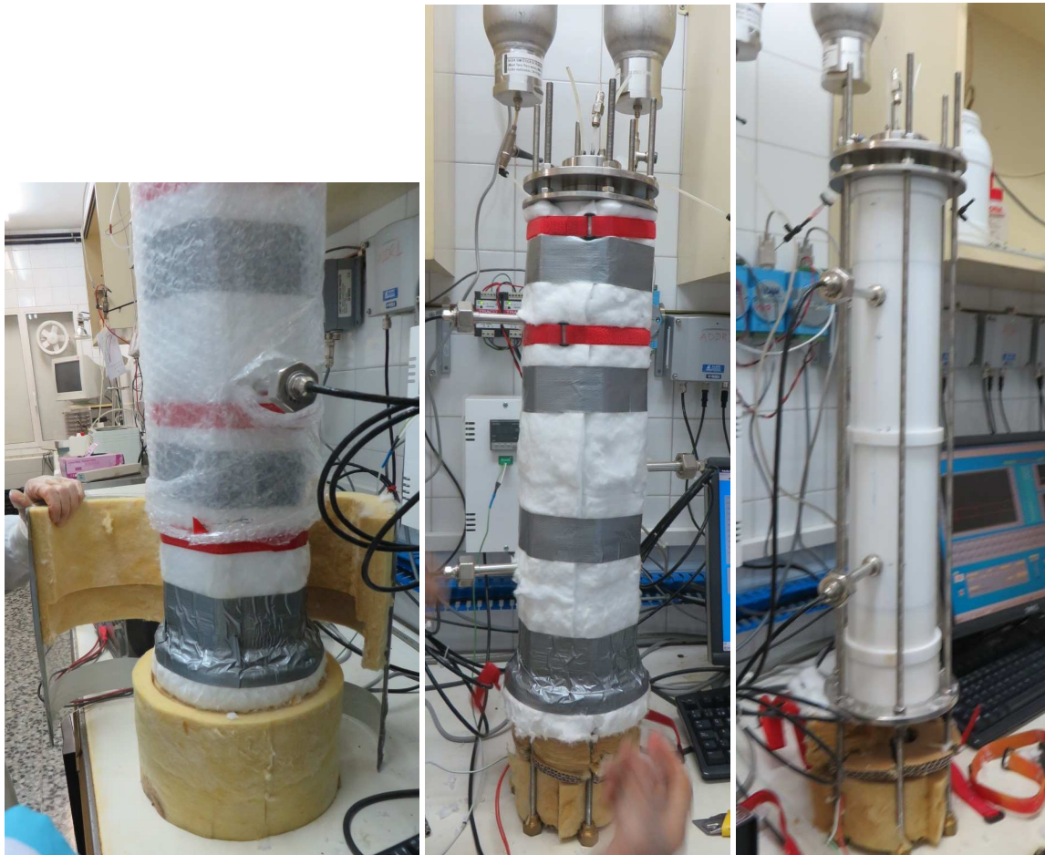
Figure 19: Removal of the isolation material
