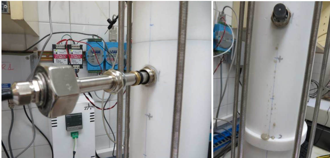
Figure 20: Extraction of sensors (left) and water drip through the sensor hole (right)
