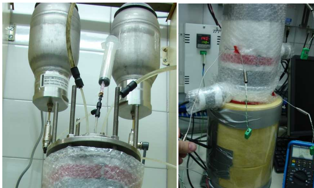
Figure 14: Hydration system with syringe connected for extracting air bubbles (left) and thermocouples installed on the cell surface and on the surface of the isolating material (right)
