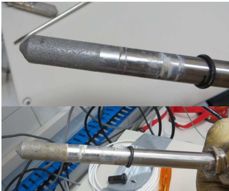
Figure 21: Appearance of sensor 1 (top) and sensor 3 (bottom) after extraction
