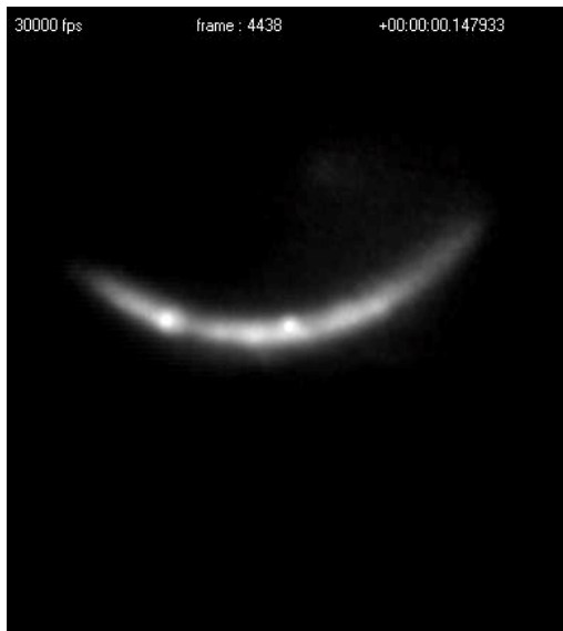
Figure 2: Dust observation in TJ-II with Li I filter, 30000 frames per second camera speed and 15 \mu s exposure time.
