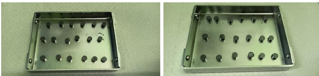
Figure 11 Photographs of the Cr-doped UO 2 pellets after sintering.
