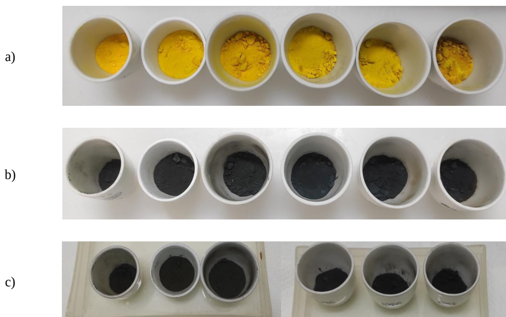
Figure 4 Photographs of the solid obtained along the co-precipitation method: a) ADU-Cr, b) U_3O_8 -Cr, and c) UO_2 -Cr. For every set of samples, Cr concentration increases from left to right.
