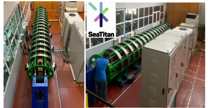
Fig. 7. Installation of the complete PTO (linear generator, power electronics and control) at the CIEMAT lab for the tests.
