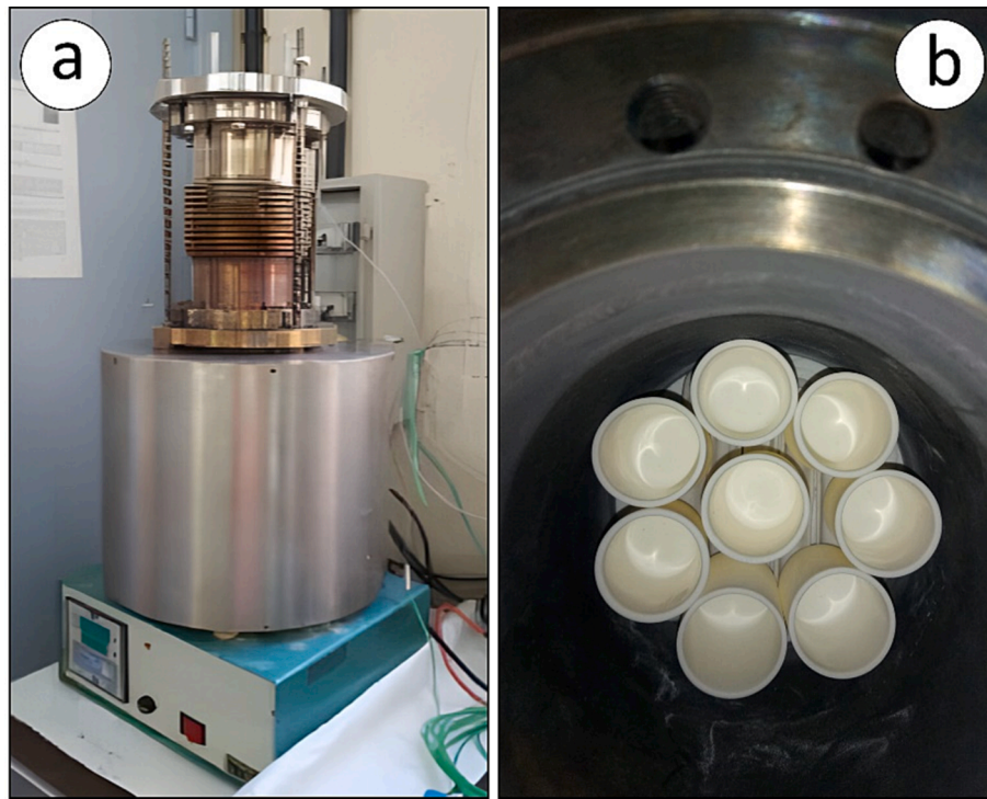
Fig. 1. (a) Image of the system where the PbLi corrosion tests were performed. (b) View of the eight high-purity alumina crucibles inside the furnace of the system where the samples were immersed in liquid PbLi for testing.
